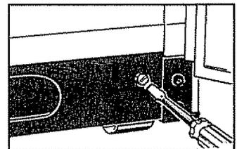
• **To replace the base grille,** line up the prongs on the grille with the clamps on the refrigerator and push forward until the grille snaps into place.
