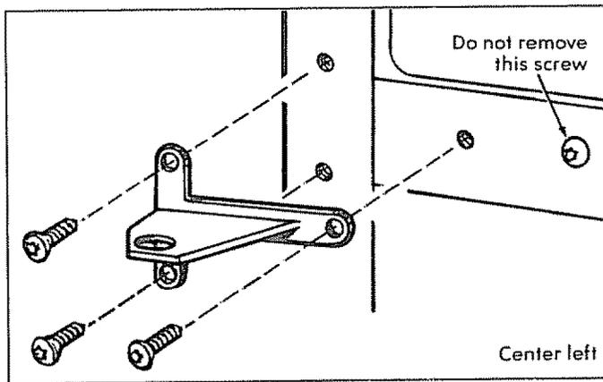
**(c)** Place the center hinge bracket over the holes at the center left side of the cabinet, insert the screws you removed from the opposite side, and tighten them.
