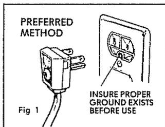
Have wall outlet and circuit checked by a qualified electrician to make sure outlet is properly grounded.
