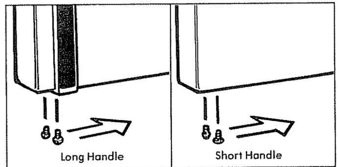
**(a)** Transfer two screws in bottom left of door to opposite side. (Wait until handle is moved before reinstalling front screw.)
