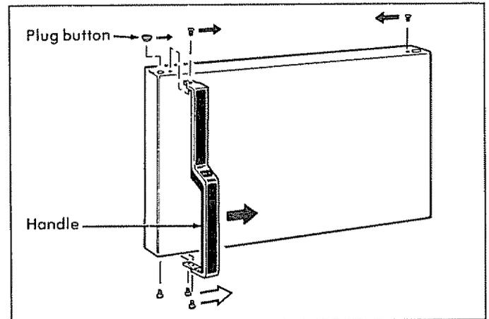
**(a)** Remove screw holding handle to top of door.
