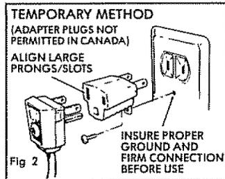
**CAUTION:** Attaching an adapter ground terminal to the wall outlet cover screw does not ground the appliance unless the cover screw is metal, and not insulated, and the wall outlet is grounded through the house wiring. You should have circuit checked by a qualified electrician to make sure the outlet is properly grounded.
