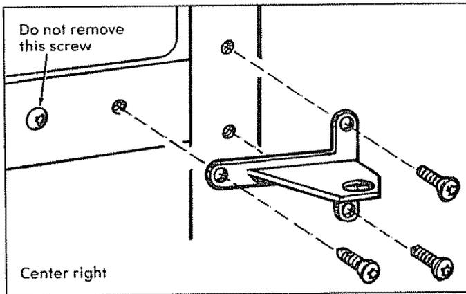
**(a)** Remove the hinge bracket (and shim glued to it) from the center right side of the cabinet by removing the three outermost Torx screws.
