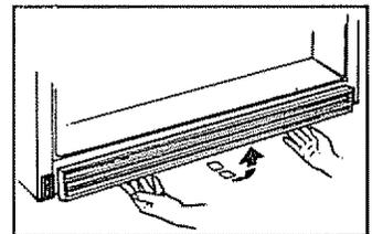
• Turn the roller adjusting screws **clockwise to raise** the refrigerator, **counter-clockwise to lower** it.
