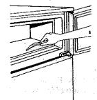
When frost is thin or soft, scrape off and remove frost on freezer compartment walls with scraper. This can be done without interrupting freezing operation.
