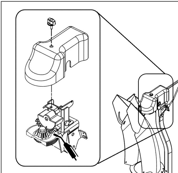
Figure 12. Lubricate Spout Rotator
