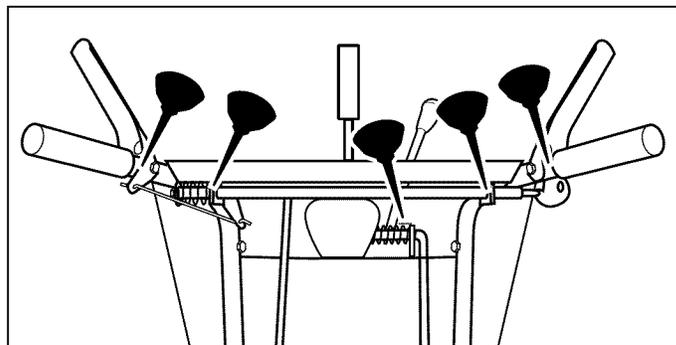
Figure 16. Lubricate Free-Hand Control
