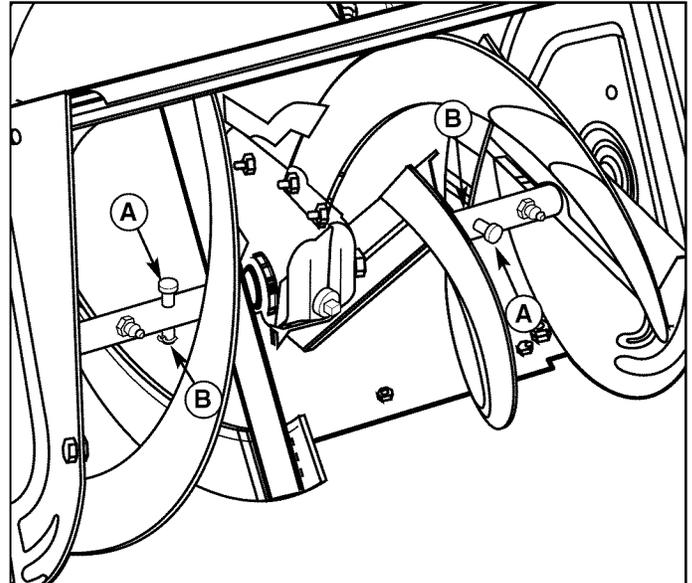
Figure 26. Shear Pins
