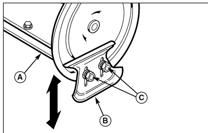
**Figure 7. Skid Shoe Adjustment**
