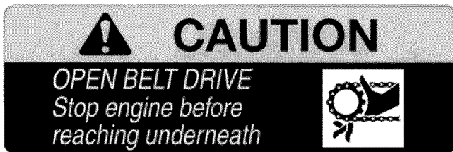
CAUTION! OPEN BELT DRIVE
