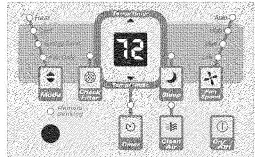
**Note:** Tap or hold either up (▲) or down (▼) button until the desired temperature is seen on the display. This temperature will be automatically maintained anywhere between 60°F (16°C) and 90°F (32°C) for cooling mode. The temperature will be automatically maintained anywhere between 55°F (13°C) and 80°F (27°C) for heating mode. If you want the display to read the actual room temperature. See "To Operate on Fan Only" section on Page 7.
