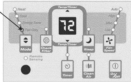
**Note:** Use this function only when cooling is not desired, such as for room air circulation or to exhaust stale air. (Remember to open the vent during this function, but keep it closed during cooling for maximum cooling efficiency.) You can choose any fan speed you prefer. (Except "Auto Fan").
