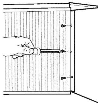
4. While the right-hand curtain is still extended, insert #10 x 1/4" pan-head Phillips screws into the top and bottom slots of curtain. Screw the curtain to the top and bottom holes in the air conditioner cabinet.
