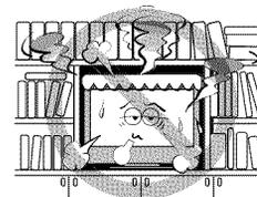
The slots and openings are provided to protect the TV from overheating and to help maintain reliable operation of the TV. Leave a space of at least 4 (four) inches around the TV.
