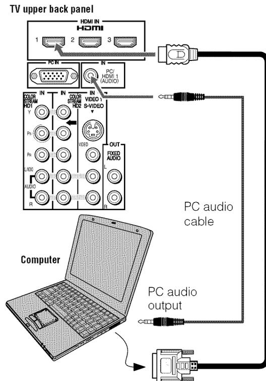
The HDMI input can accept and display VGA, SVGA, XGA, WXGA, SXGA, 480i (60Hz), 480p (60Hz), 720p (60Hz), 1080i (60Hz), and 1080p (24Hz/60Hz) signal formats. For detailed signal specifications, see page 69.
