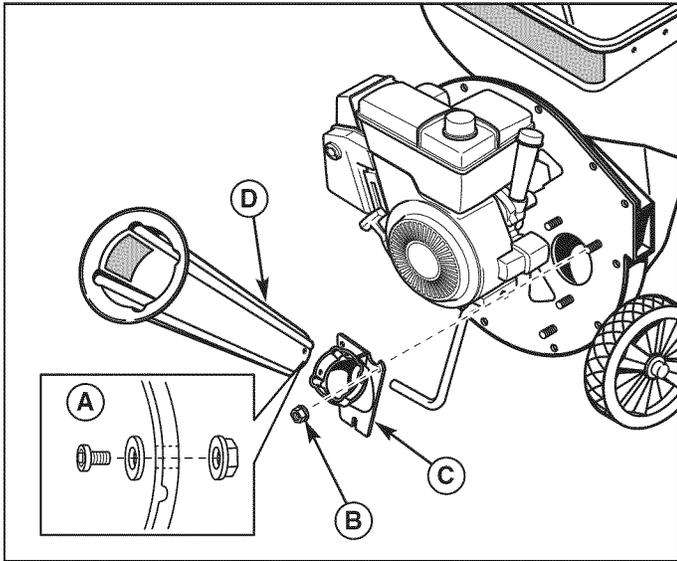
Figure 18. Installing the Chipper Cone
