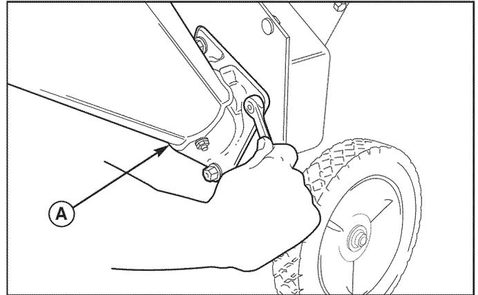
**Figure 8. Inspect Chipper Knives**
