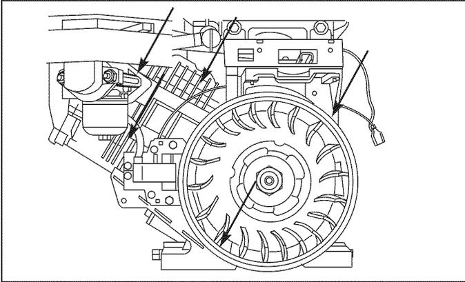
Figure 4. Clean Debris from Engine Cooling Fins
