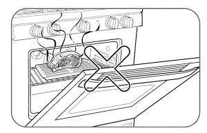
NOTE: Open door baking or broiling can cause damage to the knobs or valves. DO NOT LEAVE THE OVEN DOOR OPEN DURING COOKING OR COOL DOWN.
