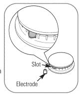
Clogged or dirty burner ports or electrodes will not allow the burner to operate properly.
