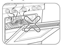
NOTE: Open door baking or broiling can cause damage to the knobs or valves. DO NOT LEAVE THE OVEN DOOR OPEN DURING COOKING OR COOL DOWN.
