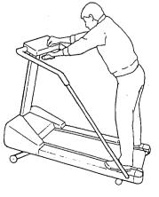
There is an Incline Indicator mounted above the Incline Control Lever on the treadmill. When the bubble in the Indicator is at level 1, the treadmill is at the lowest incline. When the bubble is at level 5, the treadmill is at the highest incline.
