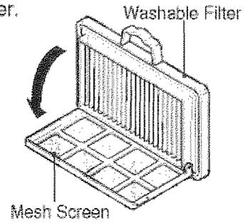
8. Clean the washable filter and the mesh screen with the brush under cold running water.
