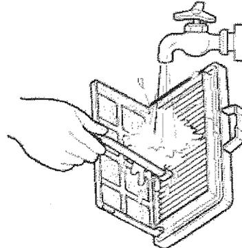
9. Allow the washable filter to dry in shaded location for a day.
