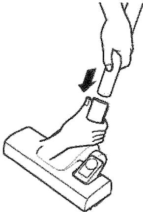
2. Push floor selector switch back for bare floor and forward for carpet. Brushes should be down for bare floor and up for carpet.
