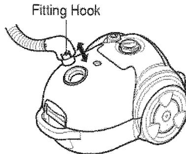
1. Insert hose into canister until it snaps into place.
