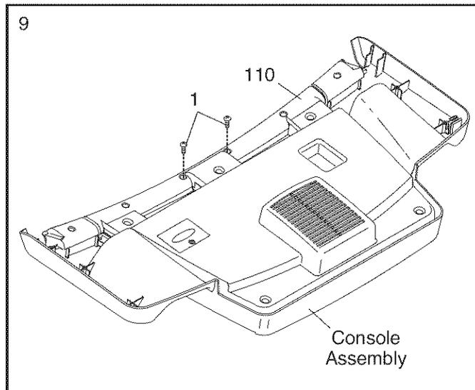
10. Set the Pulse Bar (110) on the Left and Right Uprights (77, 92). Attach the Pulse Bar with four #10 x 3/4" Screws (4) and four #10 Star Washers (12). **Start all four Screws before firmly tightening any of them. Be careful not to pinch the Wire Harness (91).**
