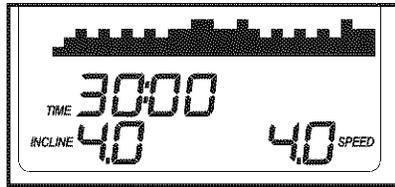
When you select a preset workout, the incline level, duration, and the speed setting will appear in the display. A profile of the speed settings of the workout will scroll across the upper half of the display.
