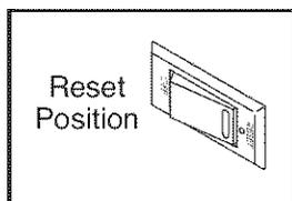
**IMPORTANT:** The console features a display demo mode, designed to be used if the treadmill is displayed in a store. If the displays light as soon as you plug in the power cord and switch the reset/off circuit breaker to the reset position, the demo mode is turned on. To turn off the demo mode, hold down the Stop button for a few seconds. If the displays remain lit, see **THE INFORMATION MODE** on page 19 to turn off the demo mode.
