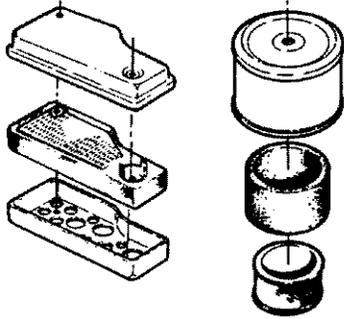
Generally, wash foam-type filters in a dishwashing detergent and water solution. Rinse and wring dry, then saturate with oil and squeeze out excess. *Failure to re-oil this type filter will ruin the engine.*
