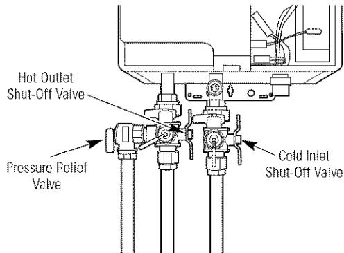
Water connections to the tankless water heater should follow all state and local plumbing codes.
