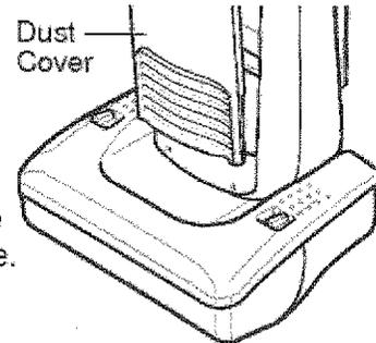
Position the dust cover so its positioning tab fits into the slot on the vacuum body base.
