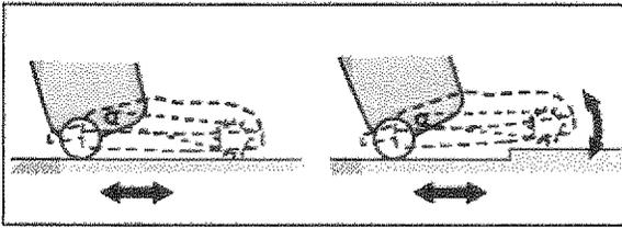
This vacuum cleaner is designed with an Automatic Height Adjustment which adjusts the floor nozzle to the proper height of any carpet pile.
