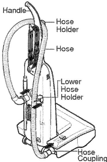
And then attach the lower hose holder provided in the accessory bag to the body and clip hose into the holder and slide hose onto the hose coupling on floor nozzle and twist hose. Make sure hose is firmly connected before using the vacuum.
