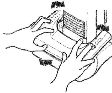
To replace nozzle cover, insert tabs into slots, lower cover onto nozzle, and push latches in to secure.
