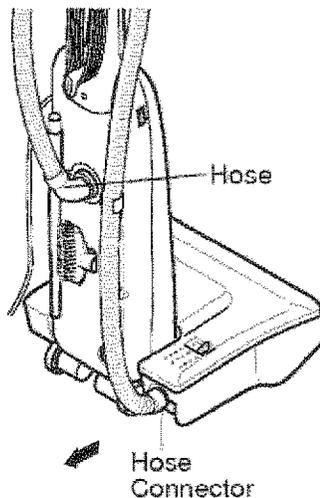
Re-insert the hose into the opening on the lower body from which it was removed. Press firmly to assure connection.
