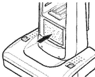
Carefully replace the dust cover by placing tabs in slots and pushing in until cover snaps into place.
