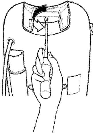
Position the handle as shown below and slide the handle into the opening at the top of the vacuum.
