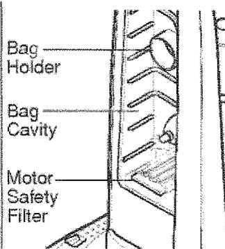
Check the bag holder and the motor safety filter.
