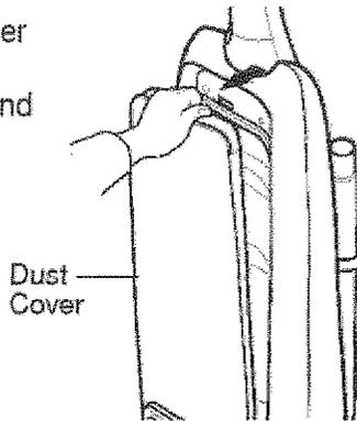
Grasp the dust bag collar and pull gently, carefully removing the dust bag.
