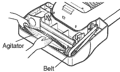
Check to see that the belt is centered on the belt pulley. Turn the agitator with your fingers to see that it turns freely.
