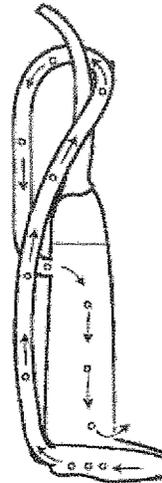
For best cleaning results, keep the airflow passage open. You should check your vacuum occasionally for clogs. The arrows in this figure indicate the airflow path where clogs occur. Unplug vacuum before checking for clogs.
