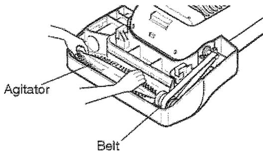
Note: It may be necessary to pull on the edge of the bumper to allow the ends of the agitator to be removed easily.
