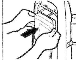
Insert the dust bag onto the bag holder completely by holding the bag collar as shown and snapping it into position.
