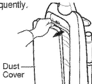
Pull the dust cover forward. Remove and lay aside.
