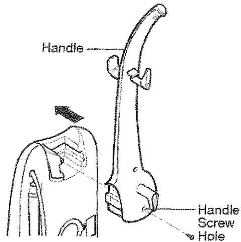
Tighten the screw securely with a screwdriver. It may be necessary to adjust the handle slightly.
