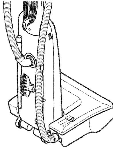
Place the crevice tool down into the extension wand. Snap wand into its storage location.
