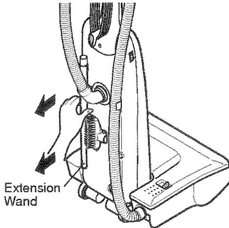
Remove the extension wand from its storage position.
