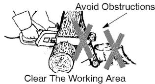
**⚠ WARNING:** Avoid kickback which can result in serious injury. **Kickback** is the backward, upward or sudden forward motion of the guide bar occurring when the saw chain near the upper tip of the guide bar contacts any object such as a log or branch, or when the wood closes in and pinches the saw chain in the cut. Contacting a foreign object in the wood can also result in loss of chain saw control.
