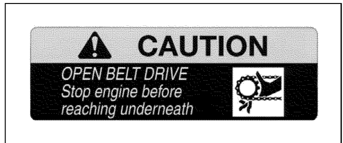
Decal - Caution - Open Belt Drive (707359) Rotating blades and other parts can cause serious injury. Keep hands and feet away.
