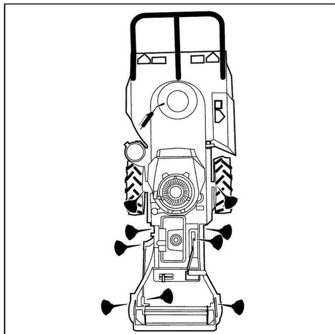
Figure 10 - Lubrication Points
