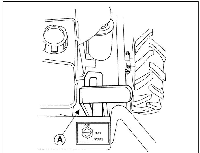
Figure 8 - PTO Disengaged
