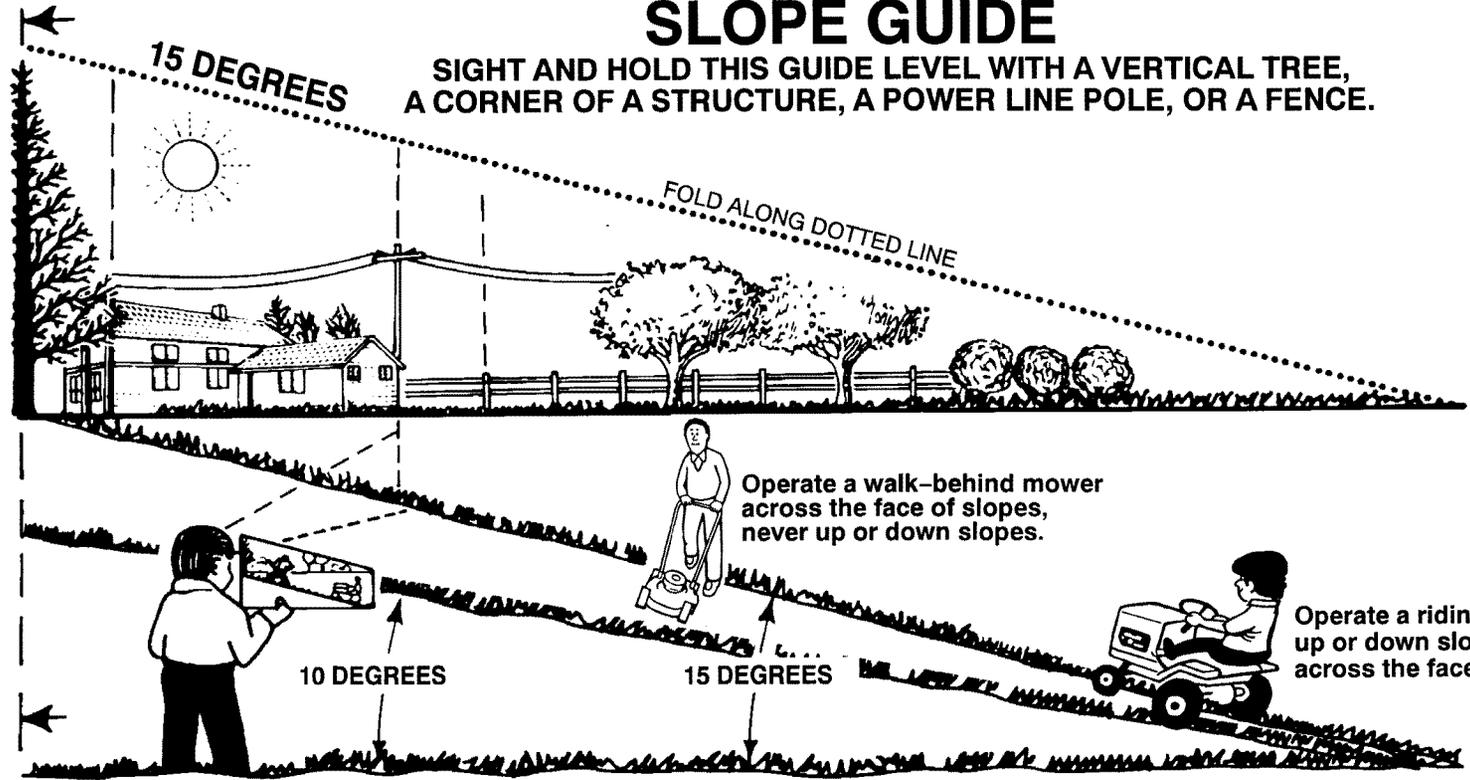
On a riding mower to determine if a slope is safe to mow: (1) disengage the blade(s), (2) put the unit in reverse, and (3) try to back straight up the slope. If you can back up the slope, it is generally safe to mow. However, if you do not feel safe, or if you are not completely sure, use this guide and do not mow a slope that is greater than 15 degrees. If the riding mower is used with a pull-behind or rear mounted attachment, do not operate the unit on a slope that is greater than 10 degrees.
