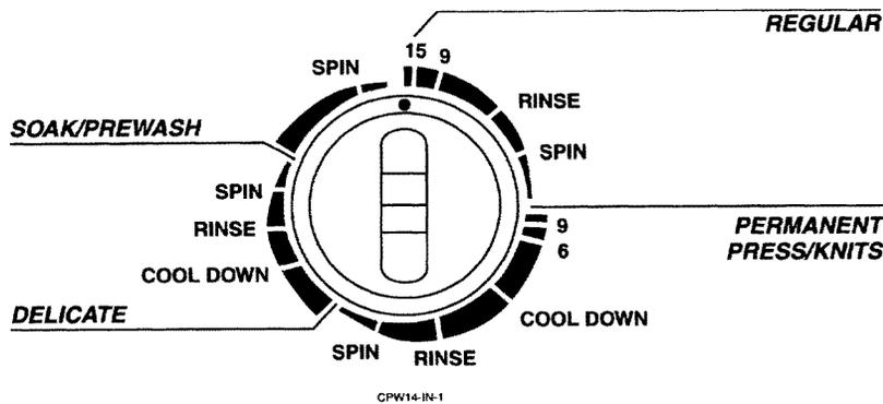
7. Select the cycle according to the type of fabric being washed. Push the timer knob in and turn clockwise to the desired cycle and wash time.
