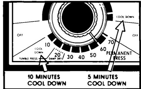
The PERMANENT PRESS Cycle has 10 minutes of cool down time at the end of the cycle.
