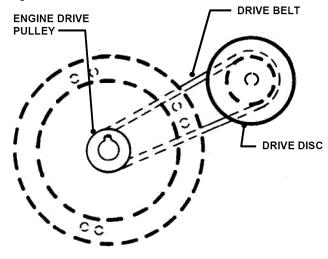
TOP VIEW OF STRETCH TYPE BELT ROUTING
