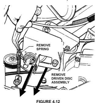
**IMPORTANT:** The bearing on these machines is staked into the thrust plate. The bearing will have to be driven out with a mallet and a large punch. A new bearing with four retaining screws will have to be purchased to replace existing bearing.
