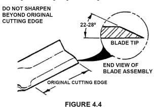
**5.** Check blade for balance. If necessary, correct balance by grinding heavy end of blade.
