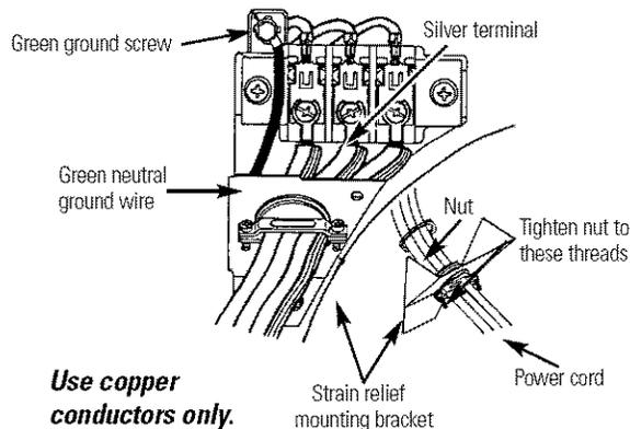
**⚠ WARNING:** Do not make a sharp bend or crimp wiring/conductor at connections.
