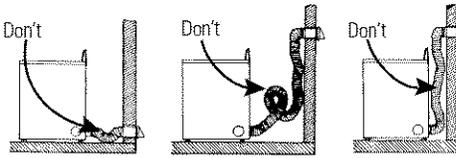
**⚠ WARNING:** The following are specific requirements for proper and safe operation of your dryer. Failure to follow these instructions can create excessive drying times and fire hazards.
