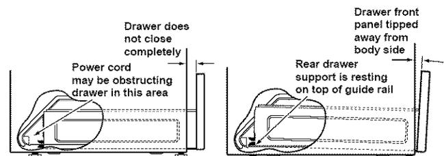
Remove and replace, making sure the power cord is not obstructing the drawer and/or the rail is in the guide.
