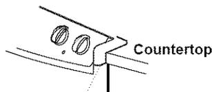
Make sure the edge of the countertop fits flush against the end of the Front Control Panel
