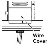
**B** Remove the knockout ring (1-3/8") located on bracket directly below the terminal block. To remove the knockout, use a pair of pliers to bend the knockout ring away from the bracket and twist until ring is removed.
