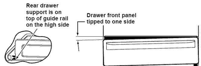
Remove and replace, making sure the rail is in the guide.
