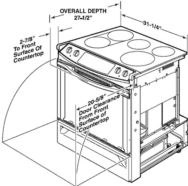
If cabinets are placed less than 30" above the range, see Alternate Construction, section AF, on page 16.
