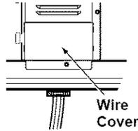
**NOTE:** When reinstalling the wire cover, make sure that wires do not become pinched between the wire cover and the housing.
