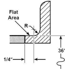
If the construction of your cabinet cannot provide a  $1\frac{1}{4}$ " flat area at the back of the countertop opening, consider changing the countertop to accommodate this dimension. See Alternate Construction section. If the area is not flat, excess tension may be applied to the glass cooktop, causing breakage and voiding the warranty.
