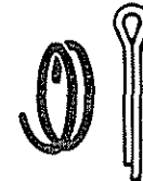
Ring or Cotter Pin Fastener (3)
