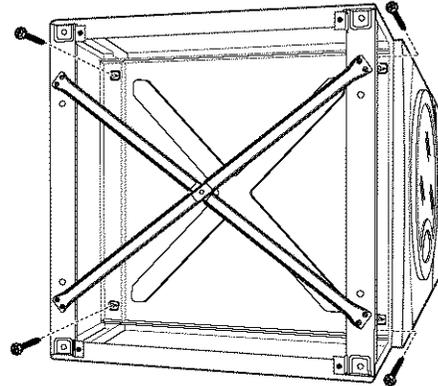
**C** Slide the pedestal toward the unit, until it is aligned front to back. Use an 8 mm socket wrench to securely tighten the screws.
