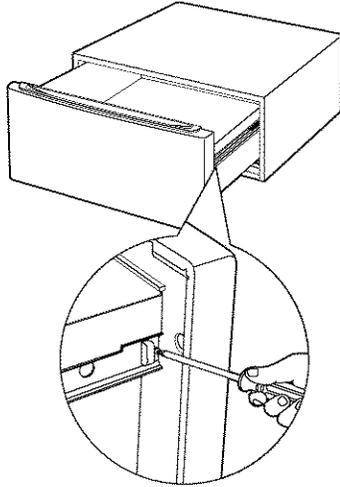
**B** Remove screws from drawer slides. Slide drawer out of the base and set aside.
