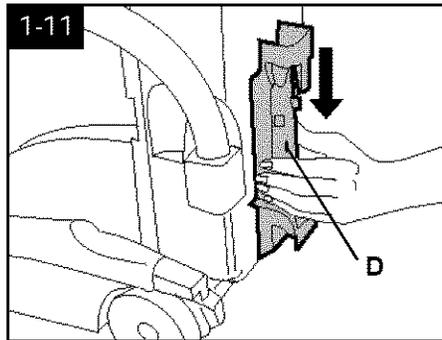
Slide rack down into place. Insert screw at (D) and tighten with a Phillips screwdriver.
