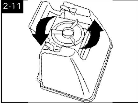
Rotate tank cap counterclockwise and lift up to remove cap.
