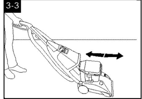
5. Squeeze trigger to release cleaning solution and **slowly** push deep cleaner forward (equals one wet stroke).
