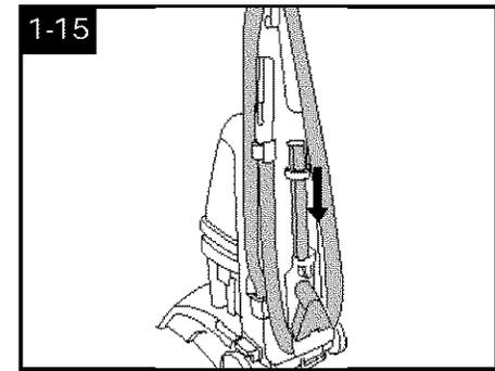
Slide bare floor attachment into holder as shown.
