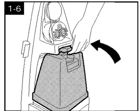
Replace clean solution tank (upper tank) by positioning bottom first. Press on tank handle to snap top of tank into place.
