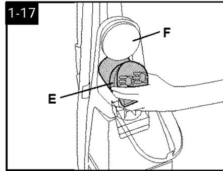
To remove powered hand tool (E), pull it down and outward.
