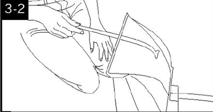
Some models have a nozzle clean-out tool for removing debris or if a non-carpeted floor is not available. To use the tool: **Disconnect deep cleaner from electrical outlet.** Slide tool into nozzle and remove debris as shown.
