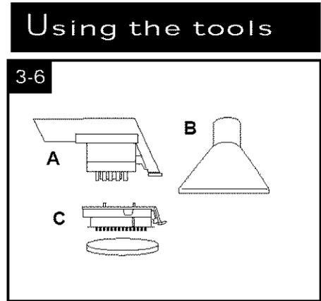
**A. Powered hand tool** has rotating brushes for extra scrubbing action on small carpet areas, carpeted stairs and upholstery. Brushes can be removed for converting to the scrub module.
