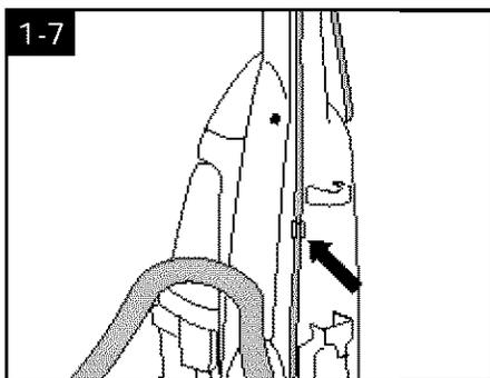
Press cord into cord clip on back of handle. Pull cord tight.
