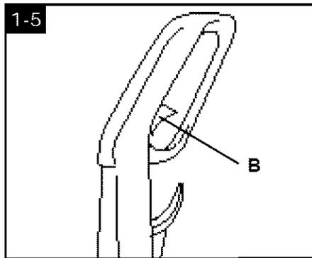
When handle sections are completely together, squeeze trigger (B) on upper handle to snap trigger rod in place.
