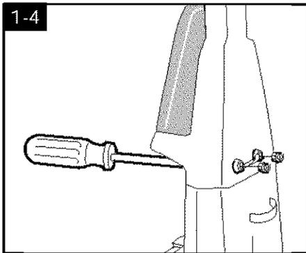
Place nuts in recessed areas on **back of handle**. Hold each nut in place while tightening each bolt securely with a Phillips screw driver.
