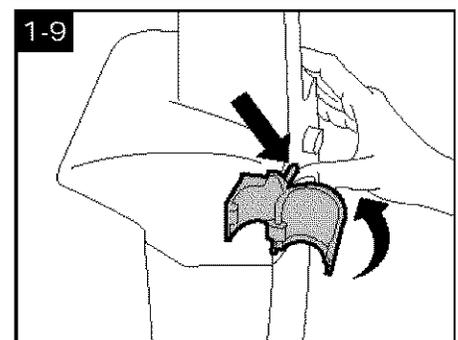
Pivot clip and push other tab into hole at back of handle to lock into place.
