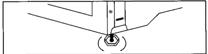
**WARNING:** To reduce the risk of accidental tipping of the range, it must be secured by an anti-tip device. To check if the device is installed properly, use a flashlight and look underneath the range to see that one of the rear leveling legs is engaged in the bracket slot. The anti-tip device secures the rear leveling leg to the floor, if properly engaged.
