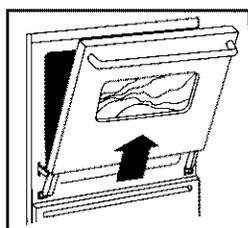
**To Replace Oven Door:** Grasp the door at each side, align the slots in the door with the hinge arms and slide the door down onto the hinge arms until it is completely seated on the hinges.
