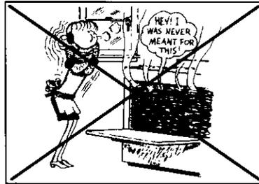
Do not obstruct the flow of combustion and ventilation air by blocking the oven vent or air intakes. Restriction of air flow to the burner prevents proper performance and increases carbon monoxide emission to unsafe levels.
