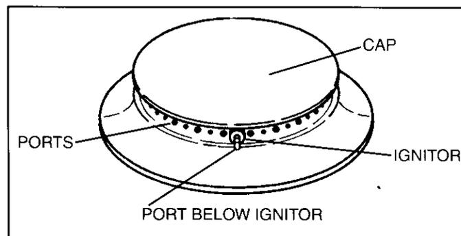
**NOTE:** The surface burner will not light if the ignitor is damaged, broken, soiled or wet. Also, the burner will not light if the small port beneath the ignitor is blocked. See pages 14-15 for cleaning instructions.
