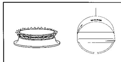
**Be sure to adjust the knob so there is an adequate supply of gas to maintain a stable flame on the burner.** Check to be sure burner is lit and the flame is stable.
