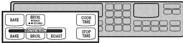
The electronic clock/oven control will turn the oven on and off at times you set, even when you are not around.
