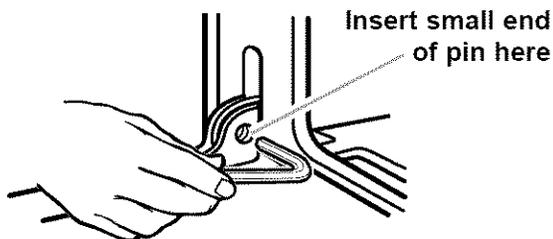
3. Grasp under handle and gently close door as far as it will shut. Pull door out at bottom to remove.
