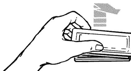
3. Remove the light bulb from its socket. Replace the bulb with another halogen bulb (12 volt, 5 watt maximum, available at most hardware stores).
