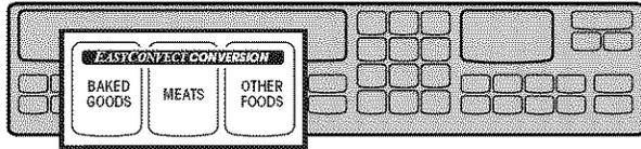
EASY CONVECT Conversion lets you convection cook without entering convection cook temperatures and times. Simply enter the standard cook temperature and time for the food to be cooked. The oven will reduce the temperature, or the temperature and time, for convection cooking. (Convection temperatures and times are not as long because the heated air is circulated in the oven cavity for quicker cooking.)
