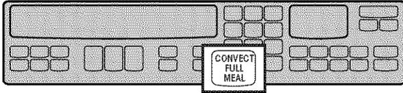
CONVECT FULL MEAL lets you choose from among ten preset oven convection cooking cycles, all using the convection fan. These cycles store commonly used cooking times, cooking temperatures, and probe temperature settings. CONVECT FULL MEAL saves you time by limiting the number of pads you have to press when cooking at a favorite setting. CONVECT FULL MEAL also lets you set your own favorite cycle (either convection or nonconvection).
