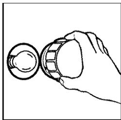
4. Replace the bulb cover by turning it clockwise.
