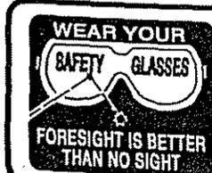
The operation of any reciprocating saw can result in foreign objects being thrown into your eyes, which can result in severe eye damage. Before beginning power tool operation, always wear safety goggles or safety glasses with side shields and a full face shield when needed. We recommend Wide Vision Safety Mask for use over eyeglasses or standard safety glasses with side shields, available at Sears Retail Stores.
