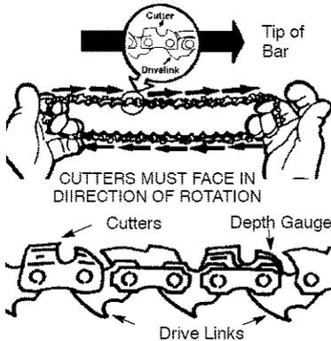
8. Place chain over and behind clutch retainer, fitting the drive links in the clutch drum sprocket.
