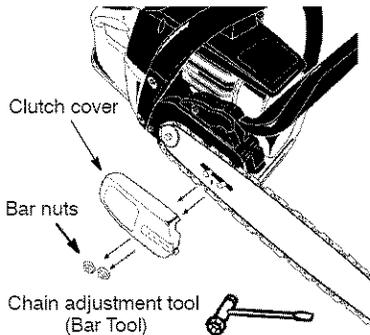
4. Turn adjusting screw on bar counterclockwise to move the tensioning rack as far as it will go toward the front of the bar.
