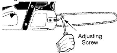
4. Using bar tool, roll chain around guide bar to ensure all links are in bar groove.
