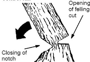
**NOTE:** Before felling cut is complete, use wedges to open the cut if necessary to control the direction of fall. To avoid
