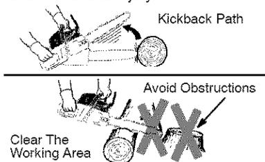
**⚠ WARNING:** Avoid kickback which can result in serious injury. **Kickback** is the backward, upward or sudden forward motion of the guide bar occurring when the saw chain near the upper tip of the guide bar contacts any object such as a log or branch, or when the wood closes in and pinches the saw chain in the cut. Contacting a foreign object in the wood can also result in loss of chain saw control.
