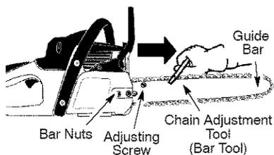
2. Loosen bar nuts until they are finger tight against the clutch cover.
