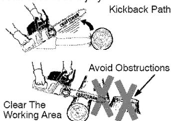
**⚠ WARNING:** Avoid kickback which can result in serious injury. **Kickback** is the backward, upward or sudden forward motion of the guide bar occurring when the saw chain near the upper tip of the guide bar contacts any object such as a log or branch, or when the wood closes in and pinches the saw chain in the cut. Contacting a foreign object in the wood can also result in loss of chain saw control.
