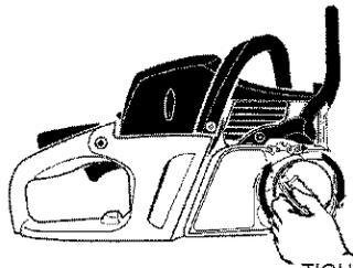
6. Push lever on bar knob down to return lever to closed/locked position.
