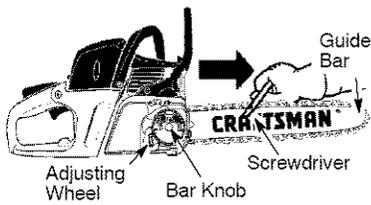
2. Lift lever on bar knob and turn counterclockwise 1 turn to loosen bar clamp.
