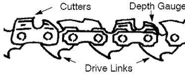
7. Place chain over and behind clutch retainer, fitting the drive links in the clutch drum sprocket.
