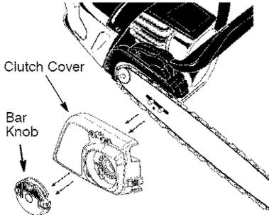
4. Slide guide bar on bar bolts until guide bar stops against clutch drum sprocket.
