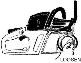
3. Loosen chain tension by turning adjusting wheel (upward direction). Remove clutch cover.
