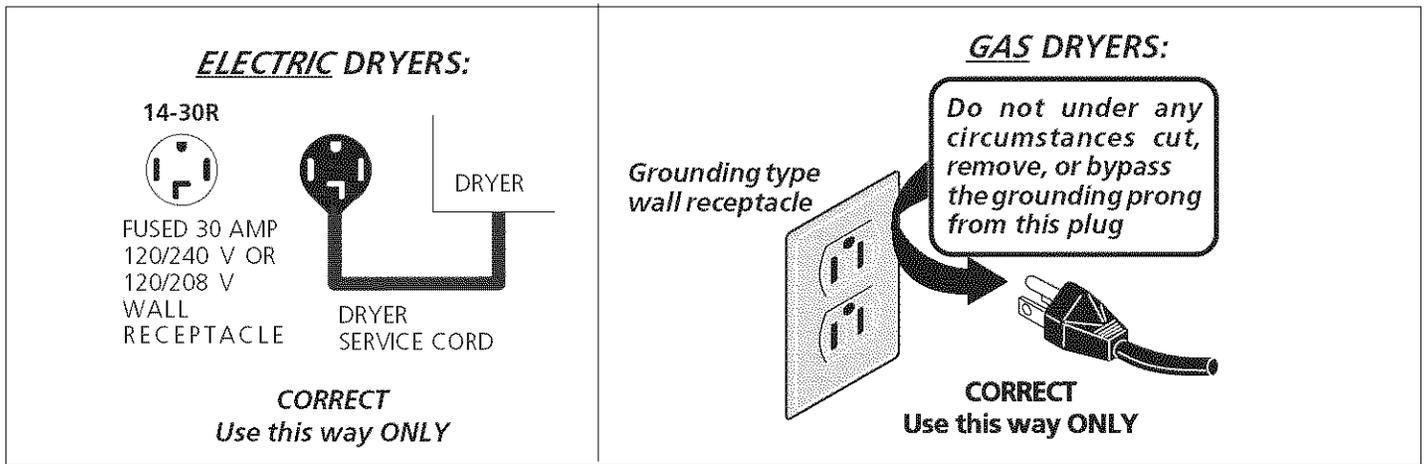
**⚠ WARNING** Avoid fire hazard or electrical shock. Do not use an adaptor plug or extension cord or remove grounding prong from electrical power cord. Failure to follow this warning can cause serious injury, fire or death.
