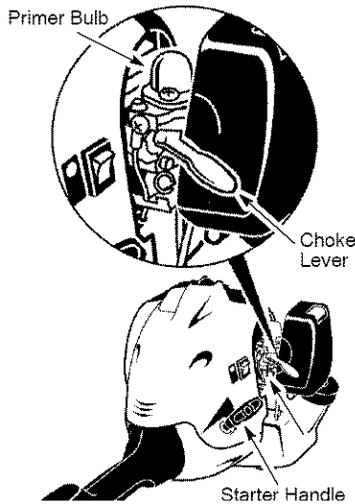
5. Pull starter rope handle sharply until engine sounds as if it is trying to start, but do not pull rope more than 6 times.
