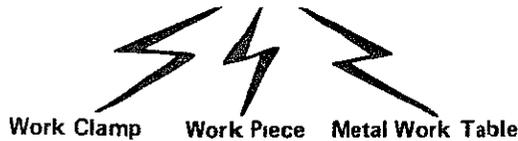
80 volts exist between these parts when welder is on!!!
