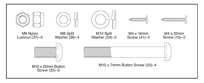
Identify the Front Stabilizer (2), which is narrower than the Rear Stabilizer (not shown). While another person lifts the front of the Frame (1), attach the Front Stabilizer to the Frame with two M10 x 74mm Button Screws (33).
