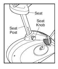
loosen it (if the knob is not loosened enough, it may scratch the seat post). Next, pull the knob, slide the seat post to the desired height, and then release the knob. Move the seat post upward and downward slightly until the pin on the knob snaps into one of the holes in the seat post. Then, turn the knob clockwise until it is tight.
