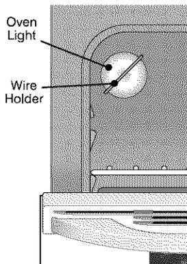
The oven light bulb is located at the rear of the oven and is covered with a glass shield held by a wire holder. The glass shield must be in place whenever the oven is in use.
