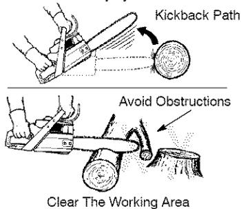
**⚠ WARNING:** Rotational Kickback can occur when the moving chain contacts an object at the upper portion of the tip of the guide bar. Contact at the upper portion of the tip of the guide bar can cause the chain to dig into the object, which stops the chain for an instant. The result is a lightning fast, reverse reaction which kicks the guide bar up and back toward the operator.
