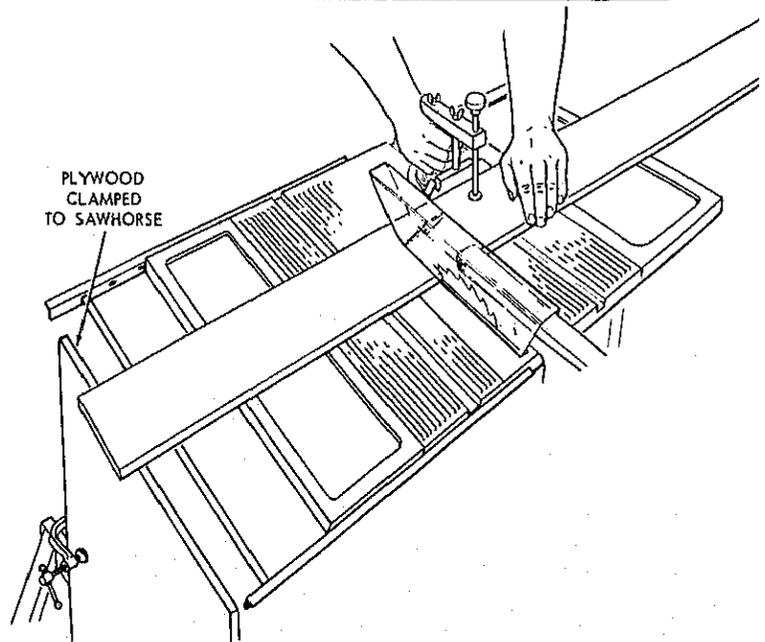
When using the RIGHT hand groove, hold the workpiece with your right hand and the lock knob with your left hand.
