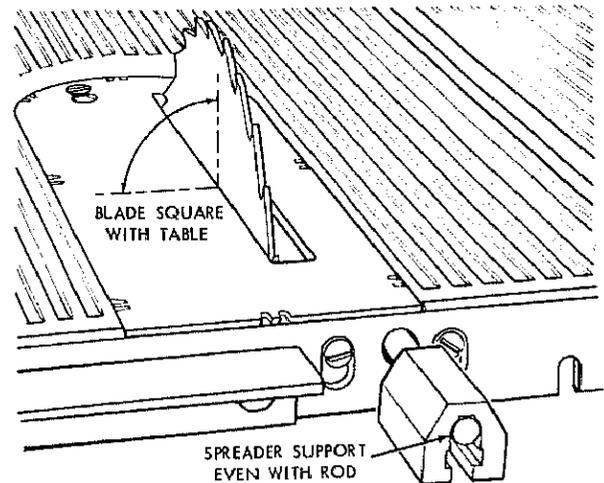
4. Assemble the 7/8 in. long setscrews, nuts, lockwashers and washers to the SPREADER SUPPORT BRACKET and slip the nuts into the slot in the spreader support.
