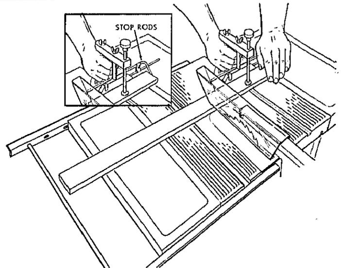
1. NEVER USE THE RIP FENCE AS A LENGTH STOP BECAUSE THE CUTOFF PIECE COULD BIND BETWEEN THE FENCE AND THE BLADE CAUSING A KICKBACK.
