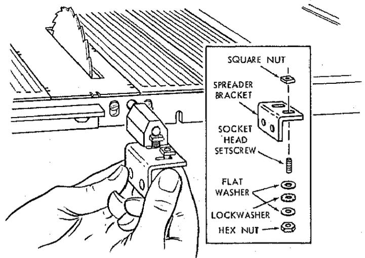
6. Lay a piece of flat straight wood and a square on saw table and rotate the SPREADER SUPPORT until the bracket is aligned with square.
