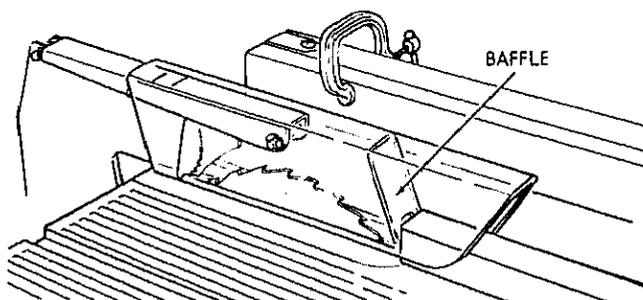
Narrow strips thicker than the Auxiliary Fence/Work Support may enter the guard and strike the baffle. CAREFULLY raise
