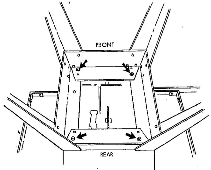
If you mount the saw on any other bench, make sure that there is an opening in the top of the bench the same size as the opening in the bottom of the saw so that the sawdust can drop through. Recommended working height is 33 to 37 in. from the top of the saw table to the floor.
