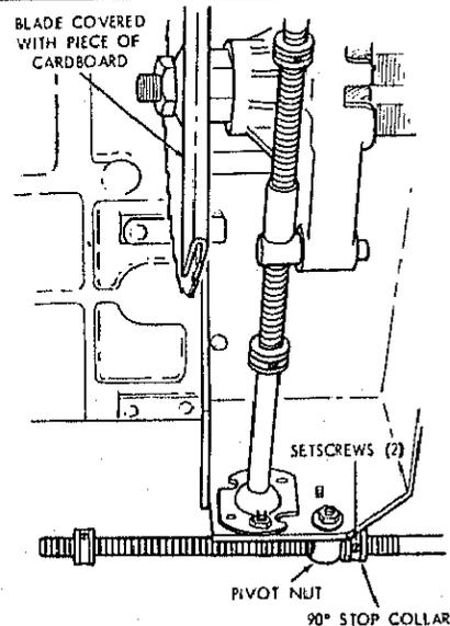
TILT blade to LEFT as far as it will go. It will stop when the PIVOT NUT is against the 45° STOP COLLAR.
