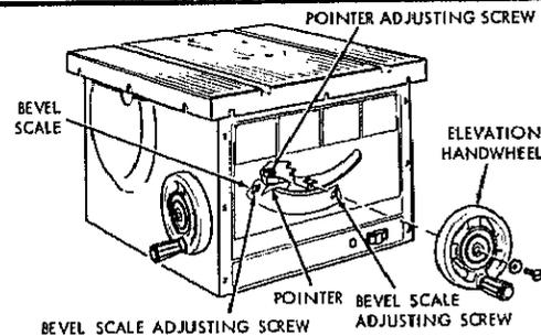
If blade is **NOT SQUARE** to table . . . the 90° **LIMIT STOP** must be **ADJUSTED**.
