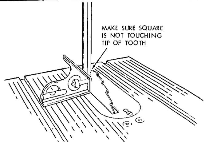
With the blade up as high as it will go, measure the distance from the top of the table to top of the highest saw tooth. If it is more than two and one half (2-1/2) inches, adjust it at this time. Refer to "BLADE ELEVATION" adjustments on page 26.
