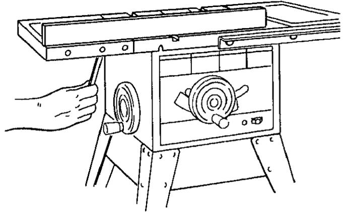
5. Hold rod with one hand and with a 1/2 in. wrench or pliers start screwing on ONE of the nuts only A TURN OR TWO . . . screw on other nut the same way. Using TWO 1/2 in. wrenches or pliers tighten both of the nuts.
