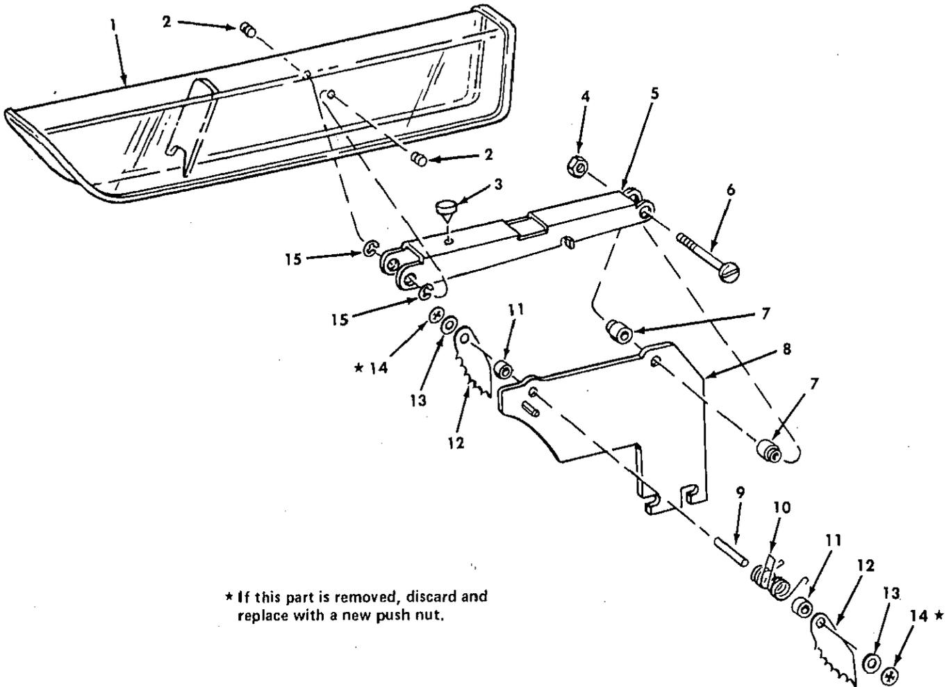
\* If this part is removed, discard and replace with a new push nut.
