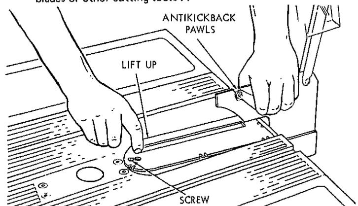
**WARNING:** FOR YOUR OWN SAFETY, TURN SWITCH "OFF" AND REMOVE PLUG FROM POWER SOURCE OUTLET BEFORE REMOVING INSERT.
