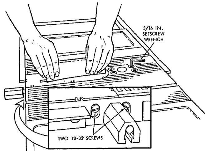
use a pair of pliers or any other tool to gain more leverage on the setscrew wrench.
