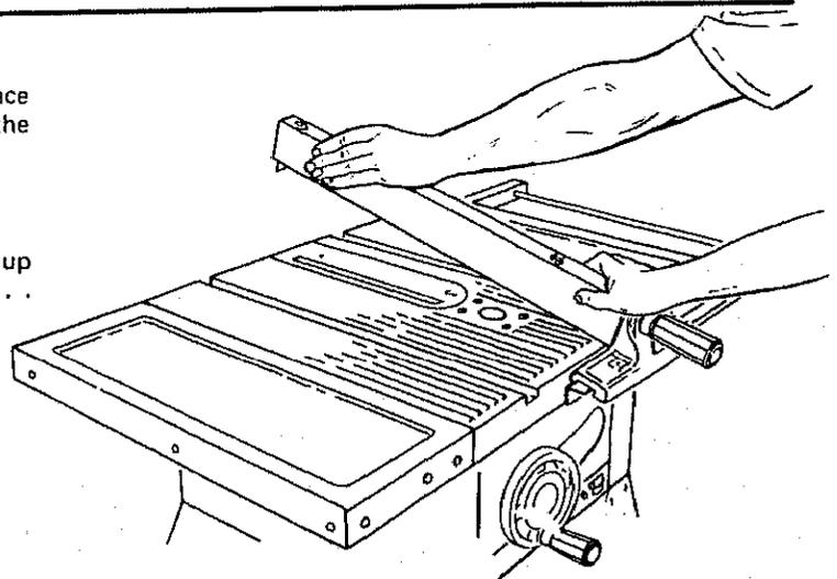
The rip fence must be PARALLEL with the sawblade and Miter Gauge grooves . . . Move fence until it is along side of groove. Do NOT LOCK IT. It should be parallel to groove. If it is not;
