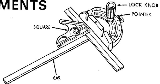
2. Position the head square with the bar . . . tighten the lock knob.
