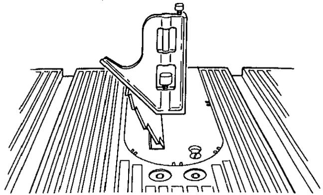
If blade is NOT 45° to table . . . the 45° STOP COLLAR and SCALE must be ADJUSTED
