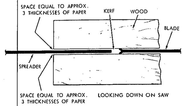
8. Make two folds in a small piece (6 x 6 in.) of ordinary NEWSPAPER making three thicknesses. The folded paper will be used as a "spacing gauge".
