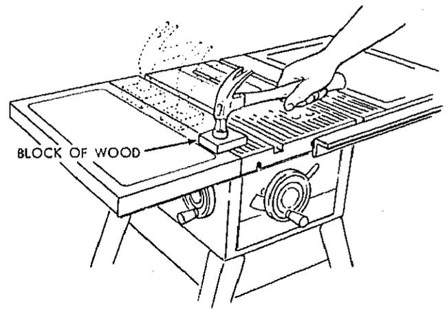
3. Lay a straight piece of wood or a framing square on table to act as a straightedge. If outer edge of extension is higher or lower than table surface:
