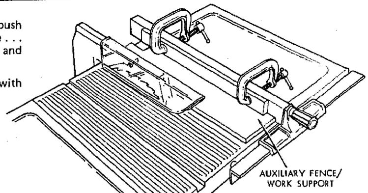
Feed the workpiece by hand along the AUXILIARY FENCE/WORK SUPPORT until the end is approx. 1 in. past the front edge of the table. Continue to feed using the PUSH BLOCK.
