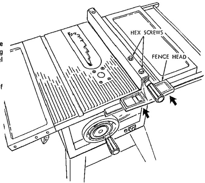
Place fence on saw but DO NOT LOCK IT. Move the REAR END of the fence slightly to the right or left . . . when you release it, the fence should "spring" back to its original position. If it does not, the spring pressure must be INCREASED.
