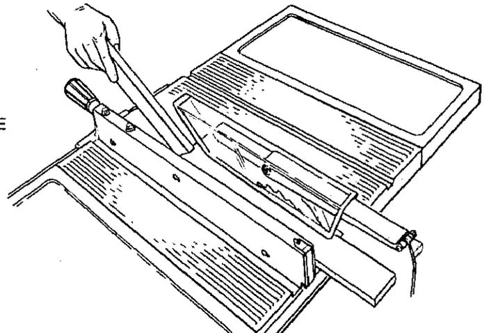
When WIDTH OF RIP is NARROWER than 2 in., the push stick CANNOT be used because the guard will interfere . . . USE the AUXILIARY FENCE/WORK SUPPORT and PUSH BLOCK.
