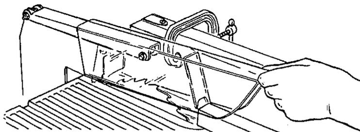
guard only enough to clear the workpiece. Use PUSH BLOCK to complete cut.
