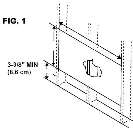
Carefully measure and cut an opening with the following dimensions depending on your model. See FIGS. 1 and 2.
