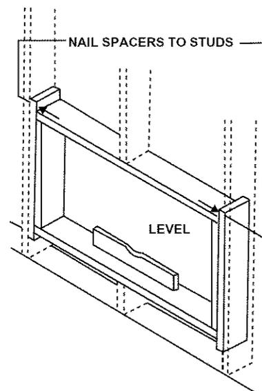
**NOTE:** If wall thickness is 8-1/2" or more, add aluminum flashing over bottom of frame opening to assure no water can enter area between inner and outer wall.
