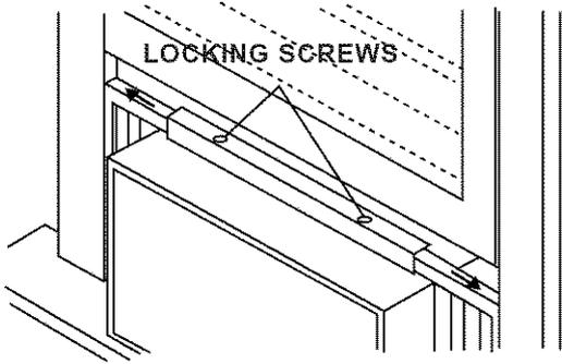
2. Extend panels to fill window opening completely. Tighten locking screws on top.
