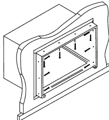
6. Install chassis into cabinet by following all steps in Step 8 of Window Mounting.(continued)
