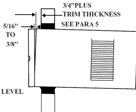
4. Secure bottom rail to wood frame with two large wood screws 1"(2.5 cm)long using the two holes in the bottom of the channel resting on frame.(See FIG.2 following)
