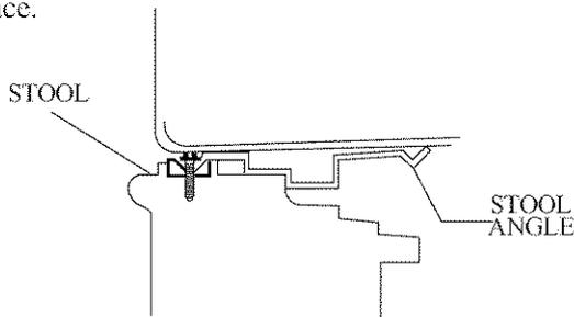
3. Shift cabinet left or right as needed to line up center of cabinet on center line marked on stool.
