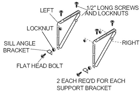
2. Assemble sill angle bracket to support brackets at the marked position, as shown. Hand tighten, but allow for any changes later.
