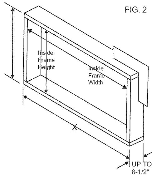
4. Build a wooden frame with the INSIDE dimensions of your model listed above. (Measure twice remember...) Frame depth should be the same as wall thickness. Fill in the space from the opening to the studs with wood spacers, as shown.
