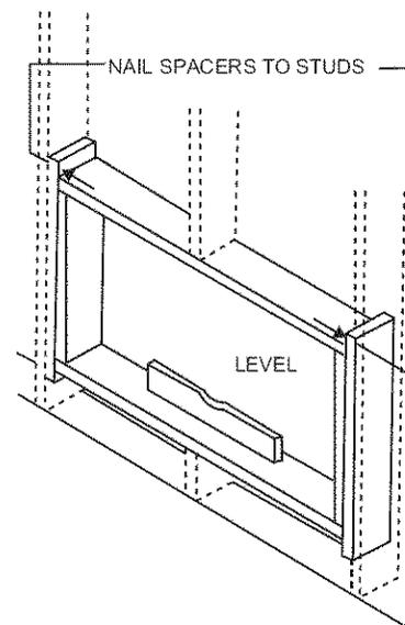
**NOTE:** If wall thickness is 8-1/2" or more, add aluminum flashing over bottom of frame opening to assure no water can enter area between inner and outer wall.
