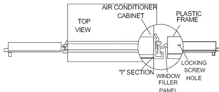
3. Insert top and bottom legs of window filler panel frame into channel in the top angle and bottom rail. Do both sides.
