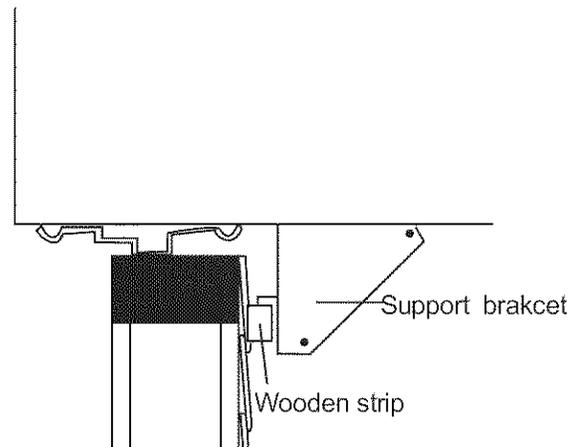
5. Screw or nail cabinet wooden frame using shims if frame is oversized, to eliminate distortion. Remember to maintain proper slope as described in Step 3.
