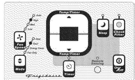
Note: This feature can be used with any combination of FAN Speeds (Low speed only on 115V models), Timer, or Sleep Modes. When in the "Heat" Mode, the fan will run continuously while heat is needed. The temperature will automatically be maintained anywhere between 55°F (13°C) and 80°F (27°C). When the room set temperature is satisfied, the fan will cycle off and on to circulate and sample the room air.
