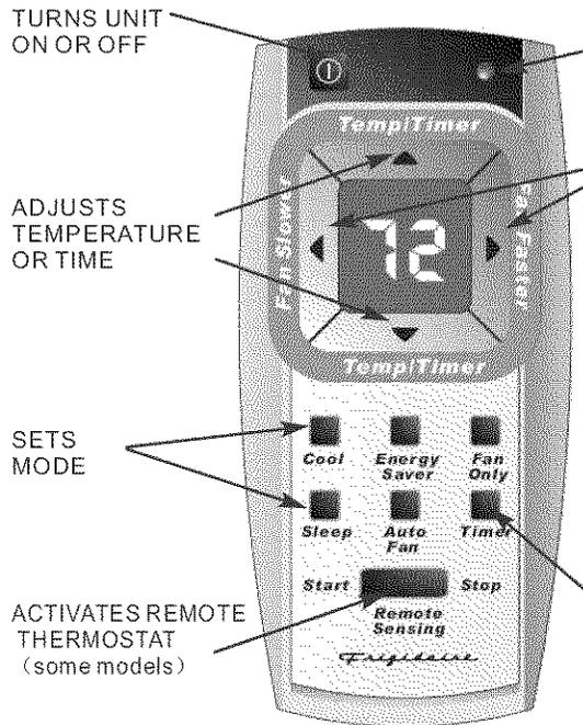
REMOTE CONTROL w/DISPLAY & REMOTE SENSING BUTTON
