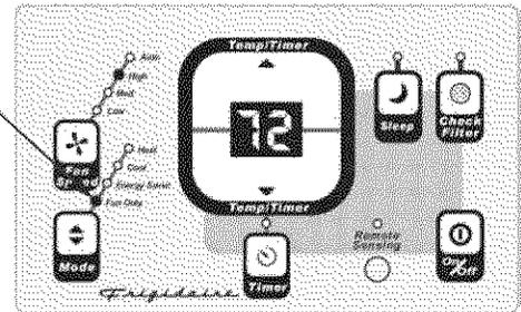
Note: Use this function only when cooling is not desired, such as for room air circulation. You can choose any fan speed you prefer, EXCEPT AUTO FAN. During this function, the display will show the actual current temperature, not the set temperature as in the cooling mode. Fan Only cannot be selected when the unit is in the 'Remote Sensing' Mode. (On those units with that feature).
