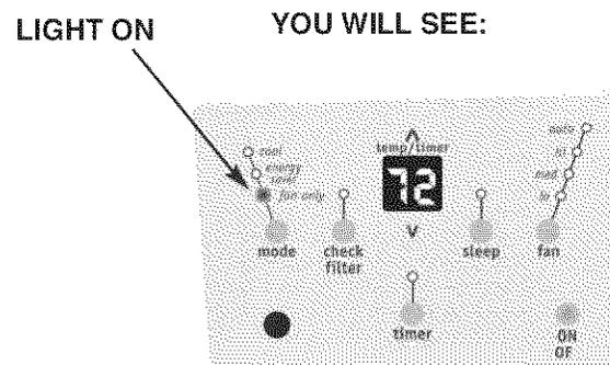
**Note:** Use this function only when cooling is not desired, such as for room air circulation or to exhaust stale air. (Remember to open the vent during this function, but keep it closed during cooling for maximum cooling efficiency.) You can choose any fan speed you prefer. (Except "Auto Fan").
