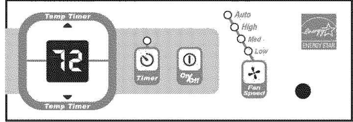
Note: Tap or hold either up(▲) or down(▼) button until the desired temperature is seen on the display. This temperature will be automatically maintained anywhere between 60°F(16°C) and 90°F (32°C). If you want the display to read the actual room temperature. See "To Operate on on Fan Only" section on Page 6.
