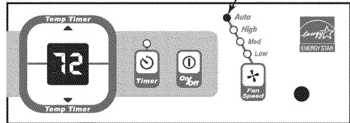
Note: Fan speed starts at high and adjusts to a slower speed as the room temperature dictates. For example, if the room doesn't get too warm it will stay at the slowest speed. If the room temperature rises quickly, such as a door being opened, it will automatically go to the highest speed. The fan speeds will rejust back to the slowest speed as the room returns to the original set temperature. Press the Fan Speed button to adjust the fan speed manually.
