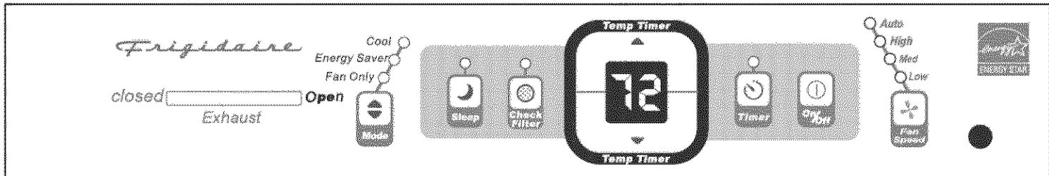
This Exhaust Control allows the air conditioner to either recirculate inside air (CLOSED) or exhaust air to the outside (OPEN). The CLOSED position is used when maximum cooling is desired. It may also be used for air recirculation without cooling When the air conditioner is set in any FAN position.
