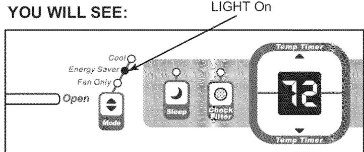
Note: In this mode, the fan will continue to run for 3 minutes after the compressor shuts off. The fan then cycles on for 2 minutes at 10 minute intervals until the room temperature is above the set temperature, at which time the unit turns back on.
