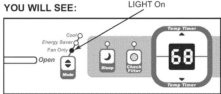
Note: Use this function only when cooling is not desired, such as for room air circulation or to exhaust stale air (Remember to open the vent during this function, but keep it closed during cooling for maximum cooling efficiency). You can choose any fan speed you prefer.
