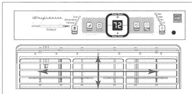
The 4-Way air directional louvers allow you to direct air flow up or down, left or right throughout the room as needed.
