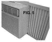
adjustments. Slide the top and bottom ends of the frame into the top and bottom rails of the cabinet. Figure 5.
