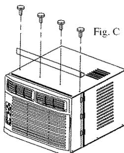
D. Secure the top rail to the unit with the 3/8" Screws as shown in Fig. C
