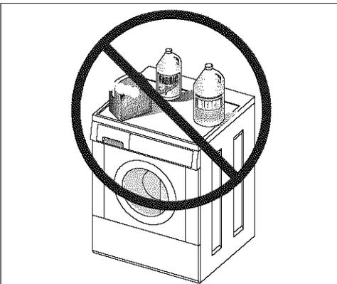
Do not store or place laundry products on top of washer at any time. They can damage the finish or controls.
