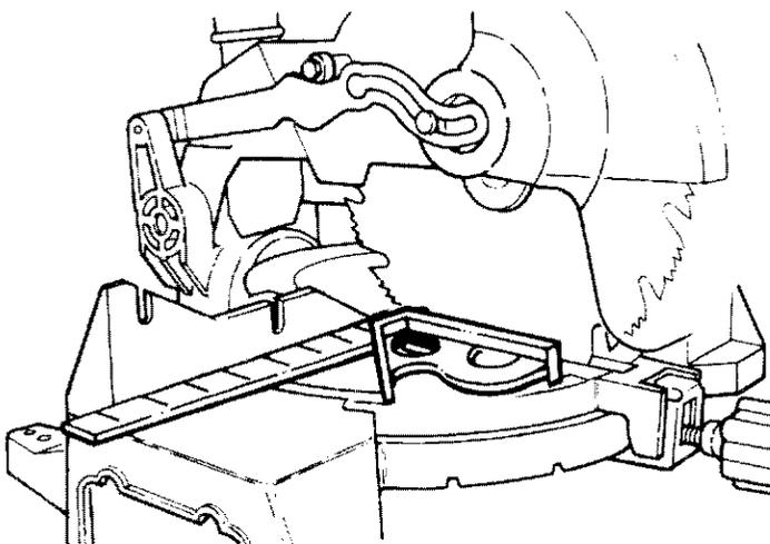
**CAUTION:** To keep from losing control of the unit, steady the base with one hand while loosening the two bolts with the other hand.
