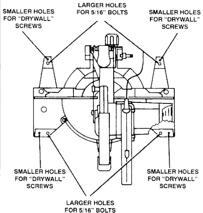
Place the saw in the desired location either on a work bench or the recommended leg set. The base of the saw has two sets of four holes to mount the miter saw, four smaller holes for "Drywall" screws and four larger holes for 5/16 bolts. (see illustration). If the saw is to be used in one location, permanently fasten it to the work bench or leg set.
