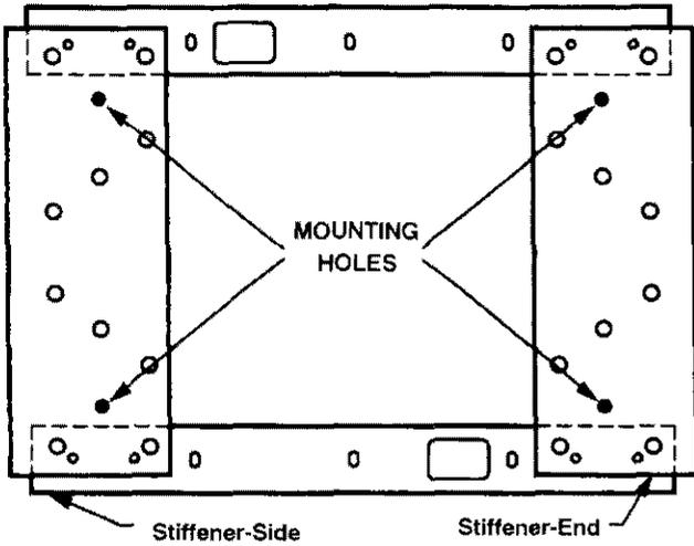
Attach miter saw to holes indicated
