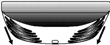
3. Replace burned-out bulb(s) with appliance bulb(s) no greater than 40 watts.
