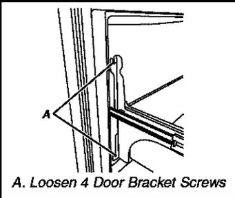
A. Loosen 4 Door Bracket Screws
